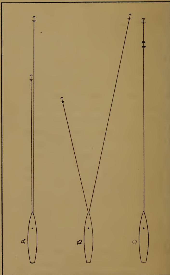
HOW TO ANCHOR WITH TWO HOOKS DOWN
